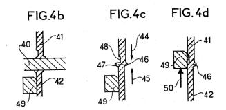
The rigid part ("starres Teil") 49, which appellant III identifies as the containing presser, is not configured for preventing the welding bead from exiting the compartment, as required by feature 11. In the method disclosed in document D18, the soft plastic compound leaves the recess 48. The rigid part 49 is then operated to spread the soft plastic compound into the
