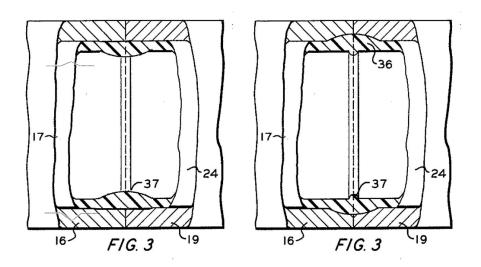
The drawing on the left showed modified containing pressers 16, 19. When the pipes 17, 24 were pressed together, all of the molten material flowed radially inwards and emerged from the groove 33. A welding bead was thus formed, which the patent intended to prevent. Therefore, the purpose and effect of the containing pressers in the drawing on the left was not to prevent welding beads. The drawing on the right, on the other
