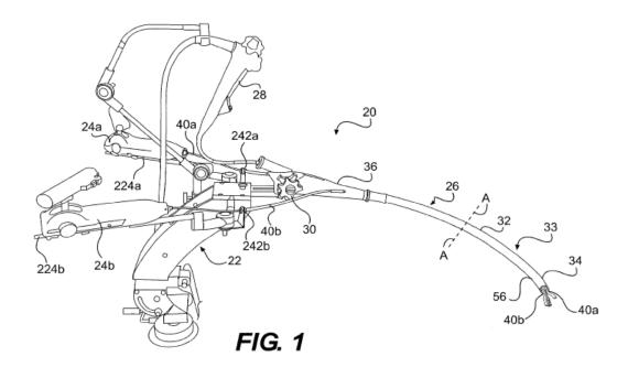
The drive system also comprises a controller (30) fixedly attached to the flexible elongate body, which can mechanically receive user input and transmit it to the distal articulation portion, for example to move the distal end of the guide tube laterally and/or up/
