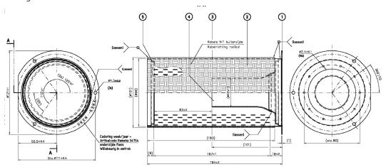
Secondly, the element (4) of E13 corresponds to an internal distributor excluded according to feature 12 ("the premixed burner does not comprise an internal distributor for distributing the air-gas mixture into the burner"). This is the case because the element (4) is arranged clearly within the tubular body (being thus "internal") and plays a role in the air-gas mixture distribution. The role in distributing the air-gas mixture is confirmed by the respondents' submission
