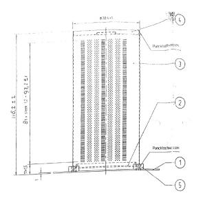
Furthermore, making the disk and flange of E6.3 integral would mean that the same resulting ensemble as shown in the document should be produced. As the respondents argued, the upper figure of E6.3 does not show any open spaces at the connection between disk and flange. Consequently, making the disk (2) integrally with the flange (1) would imply producing a continuous connection between the two parts of the ensemble to imitate the relative positions shown in E6.3.
