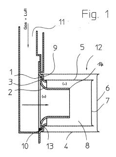
Furthermore, E9 discusses the importance of arranging free spaces ("Kurzschlussöffnungen" 1) around the head of the tubular body to compensate for pressure waves during work (see [0015] and [0016]). This suggests against closing the head of the burner in a more complete way as would be the case when replacing the funnel-shaped pipe of Figures 1 and 2 comprising a large central opening with a disk made integral with a flange.
